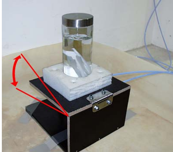
Fig 2. Agitating test performed by a tilting motion.
