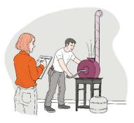
When test-running the ventilation unit the filter must not be connected.
